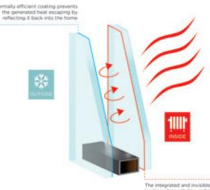
The integrated and invisible heating glass solution radiates heat into the home
