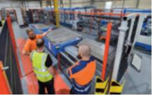
"We are continually improving our processes and embracing new technology, such as our new machining centre and scan stations. These have enabled us to automate the recording of relevant compliance information such as weld strength tests rather than relying on someone to manually check and record the information. ln fact. operators can't move forward in production unless everything meets the necessary standards. Compliance and quality are built into every step."
