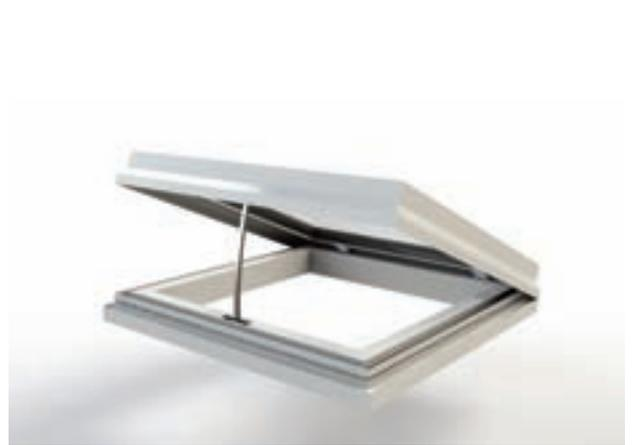
In addition, the system has been designed to allow glass to be removed in the event of a double glazed unit failure. Using a removable PVC cassette to which the glass is bonded, it is mechanically fixed to the frame, meaning only the cassette would need replacing. [i](#)
